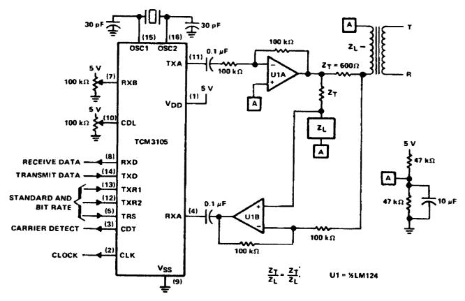
FIGURE 4. SIMPLIFIED TELEPHONE LINE INTERFACE CIRCUIT
