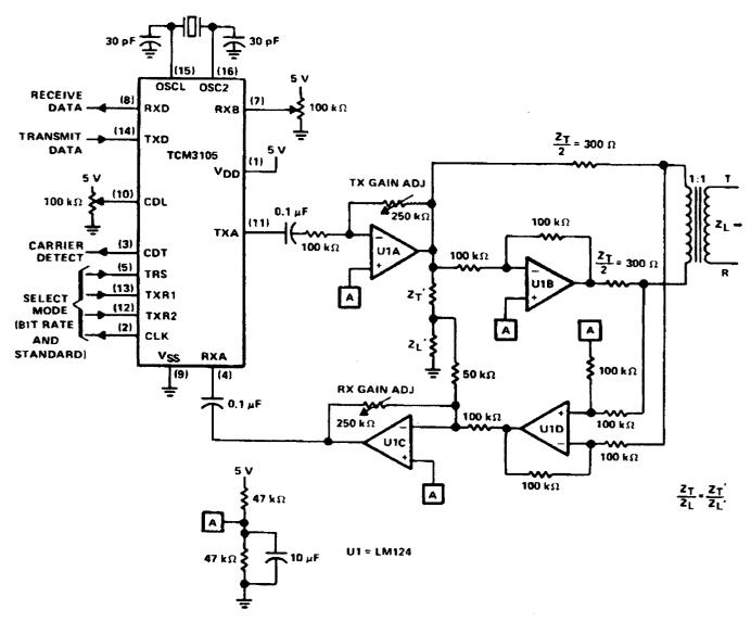
FIGURE 3. TELEPHONE LINE INTERFACE CIRCUIT
