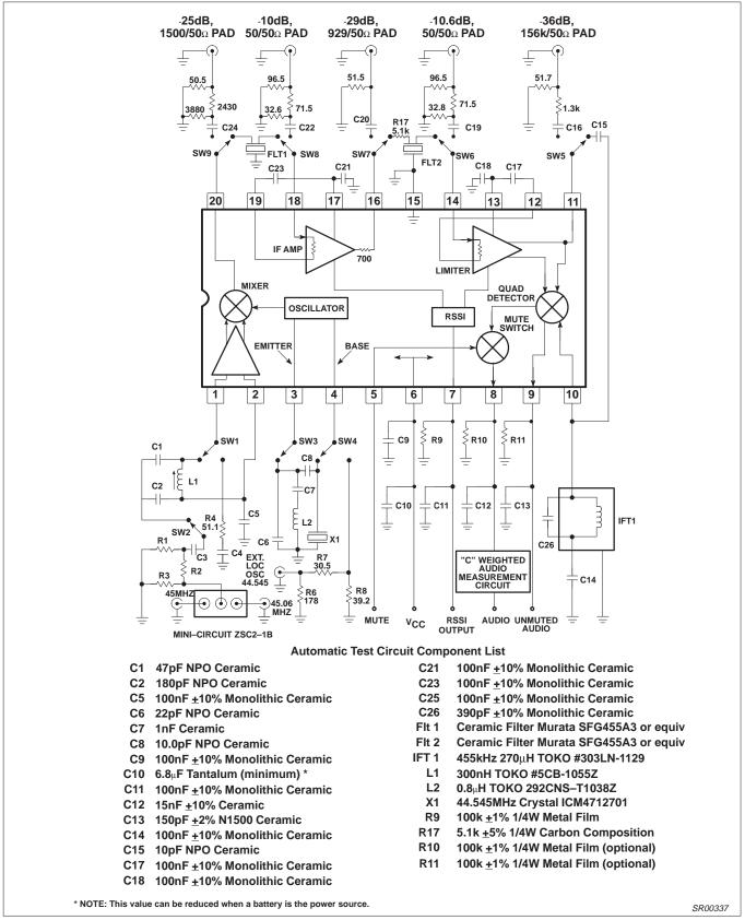
Figure 3. SA605 45MHz Test Circuit (Relays as shown)
