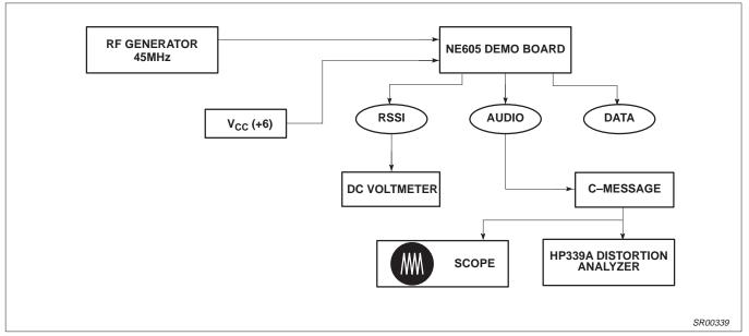
Figure 5. SA605 Application Circuit Test Set Up
