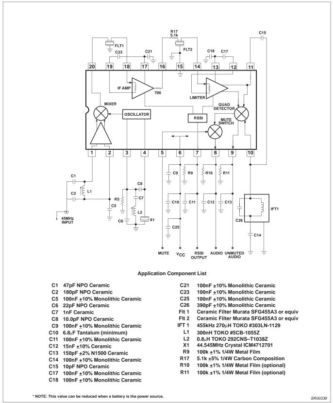
Figure 4. SA605 45MHz Application Circuit
