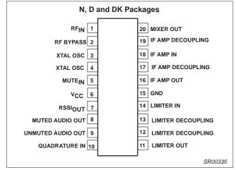
Figure 1. Pin Configuration
