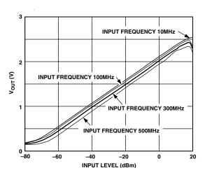
TPC 5. V<sub>OUT</sub> vs. Input Level (dBm) at Various Frequencies
