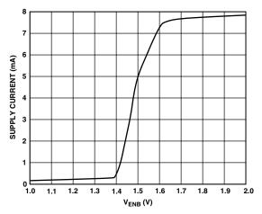
TPC 1. Supply Current vs. V<sub>ENB</sub> Voltage (5 V)
