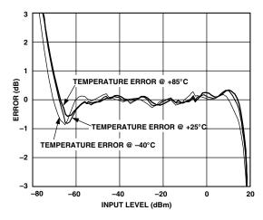
TPC 4. Log Conformance vs. Input Level (dBm) at  $+25^{\circ}$ C,  $+85^{\circ}$ C,  $-40^{\circ}$ C
