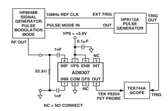
TPC 18. Test Setup for V<sub>OUT</sub> Pulse Response
