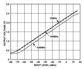
Figure 13. Log Response at 10 MHz, 100 MHz, and 500 MHz
