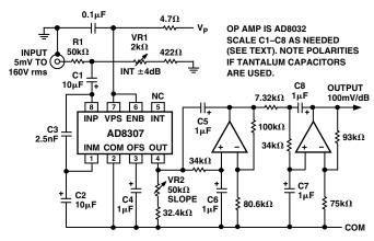
Figure 20. Log Amp with Four-Pole Low-Pass Filter
