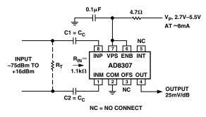
Figure 12. Basic Connections
