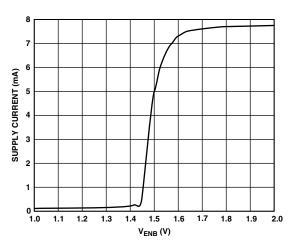
TPC 2. Supply Current vs. V<sub>ENB</sub> Voltage (3 V)
