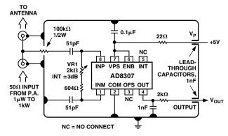
Figure 21. 1  $\mu$ W to 1 kW 50  $\Omega$  Power Meter
