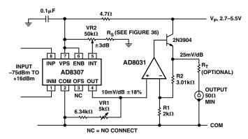
Figure 19. Cable-Driving Log Amp
