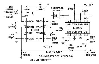
Figure 22. 120 dB Measurement System
