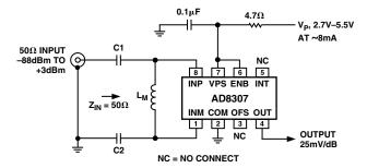
Figure 15. High Frequency Input Matching Network
