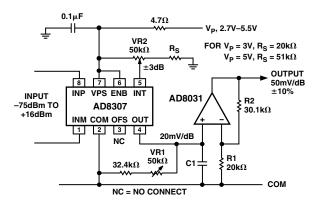
Figure 18. Log Amp with Buffered Output
