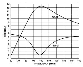
Figure 16. Response of 100 MHz Matching Network
