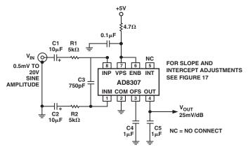
Figure 24. Connections for Low Frequency Operation
