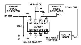
TPC 15. Test Setup for Power-Up/Power-Down Response Time
