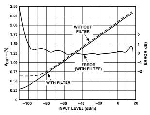
Figure 23. Results for 120 dB Measurement System
