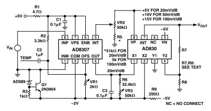
Figure 25. Connections for DC-Coupled Applications
