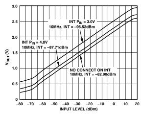
TPC 7.  $V_{OUT}$  vs. Input Level at 5 V Supply; Showing Intercept Adjustment
