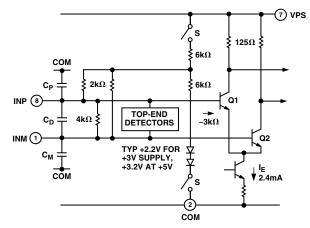
Figure 9. Signal Input Interface
