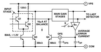
Figure 10. Offset Interface and Offset-Nulling Path
