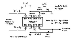
Figure 17. Slope and Intercept Adjustments
