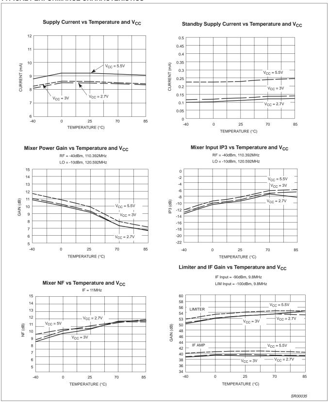
Figure 6. Typical Performance Characteristics
