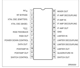
Figure 1. Pin Configuration
