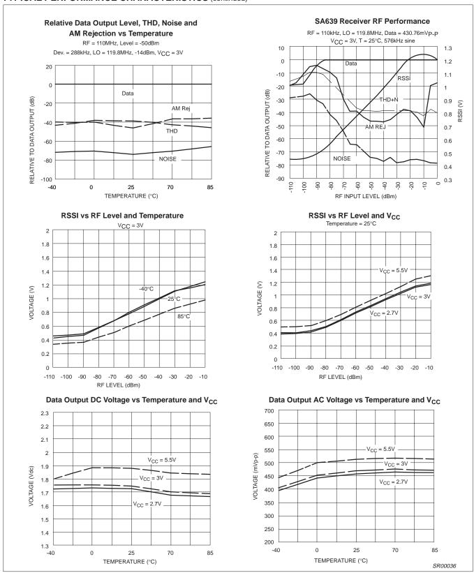
Figure 7. Typical Performance Characteristics (cont.)
