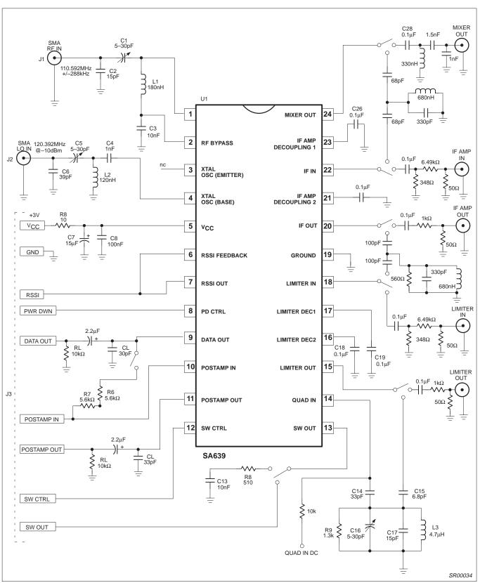
Figure 5. SA639 Test Circuit
