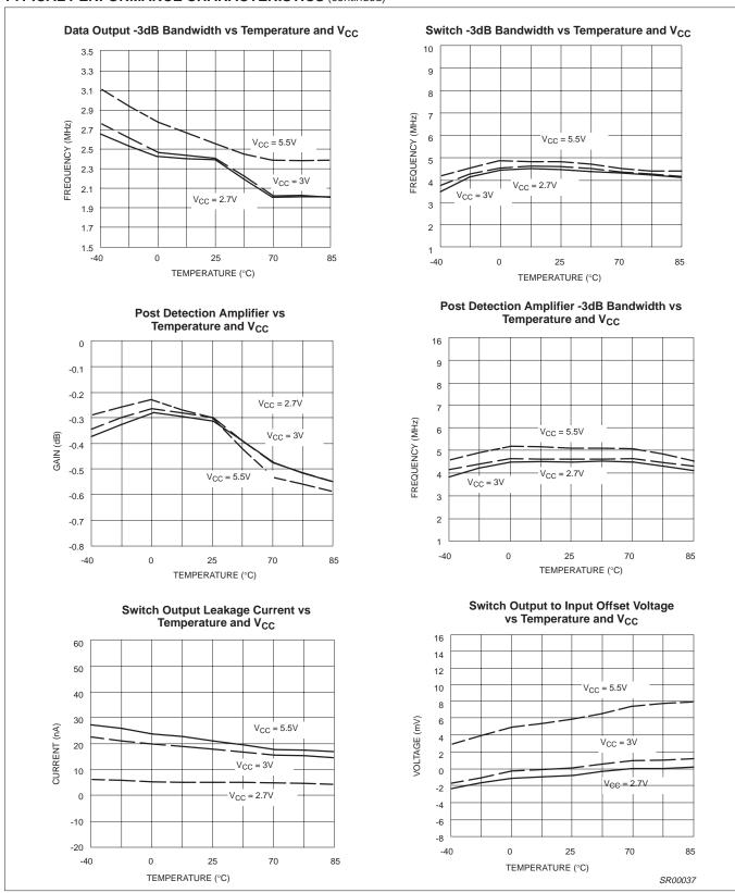
Figure 8. Typical Performance Characteristics (cont.)
