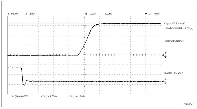
Figure 12. SA639 Data Switch Activation Time
