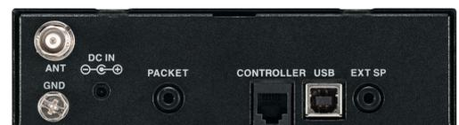
"Controller" connector is not available in the IC-PCR1500.
