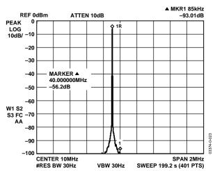
Figure 11.  $F_{OUT} = 10$  MHz, FCLK = 400 MSPS, NBSFDR,  $\pm 1$  MHz
