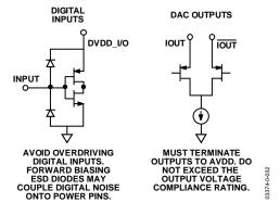
Figure 2. Equivalent Input and Output Circuits
