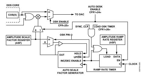
Figure 20. On-Off Shaped Keying Block Diagram
