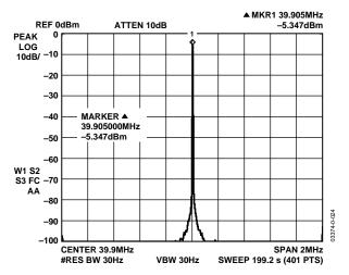
Figure 12. F<sub>OUT</sub> = 39.9 MHz, FCLK = 400 MSPS, NBSFDR, ±1 MHz
