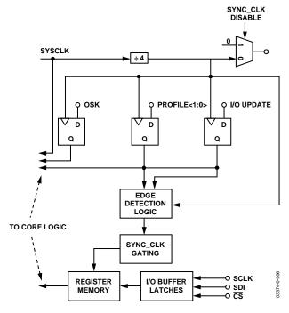
Figure 21. I/O Synchronization Block Diagram
