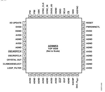
Figure 3. 48-Lead TQFP/EP
