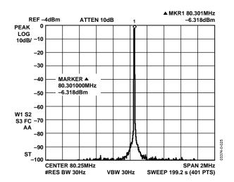
Figure 13.  $F_{OUT}$  = 80.3 MHz, FCLK = 400 MSPS, NBSFDR,  $\pm 1$  MHz
