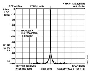
Figure 14. F<sub>OUT</sub> = 120.2 MHz, FCLK = 400 MSPS, NBSFDR, ±1 MHz
