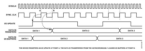
Figure 22. I/O Synchronization Timing Diagram
