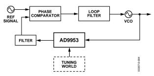
Figure 28. Digitally Programmable Divide-by-N Function in PLL
