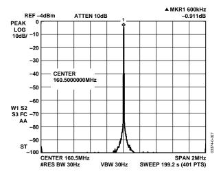
Figure 15. F<sub>OUT</sub> = 160 MHz, FCLK = 400 MSPS, NBSFDR, ±1 MHz
