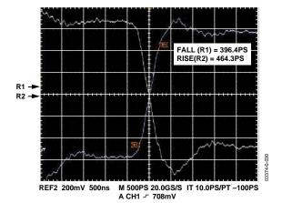
Figure 19. Comparator Rise and Fall Time at 160 MHz
