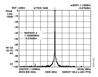
Figure 10.  $F_{OUT} = 1.1$  MHz, FCLK = 400 MSPS, NBSFDR,  $\pm 1$  MHz
